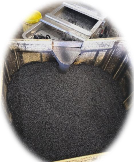
5. Pelletising extruded HDPE plastic
