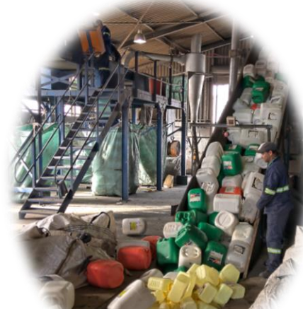
3. Triple rinsed empty HDPE containers on a conveyor on their way cleaning and shredding
