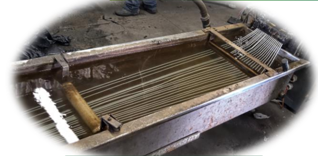
4. Molten HDPE plastic being extruded
