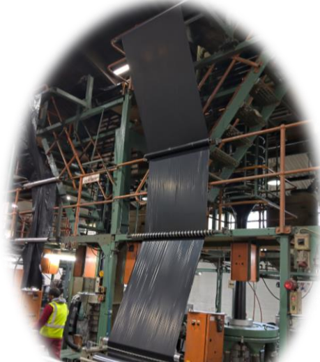
6. Manufacturing plastic refuse bags from recycled HDPE
